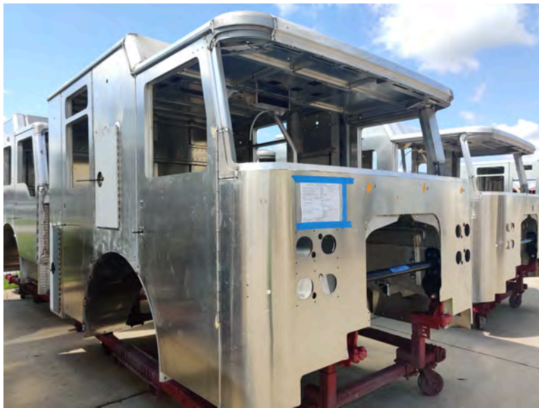
EDH Fire Engines 84 & 86 under construction at Pierce Mfg Factory in Appleton Wisconsin, July 4th 2021.
