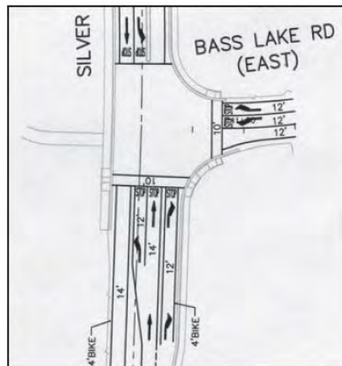
Close up view new Silver Springs Parkway-Bass Lake Road Intersection
