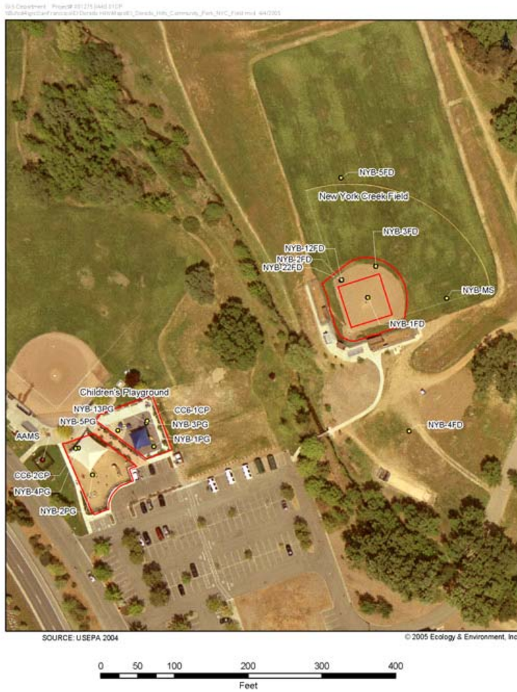
Figure 5-14 Community Park New York Creek Field Activity-Based Outdoor Air Sampling Locations Baseball Scenario
