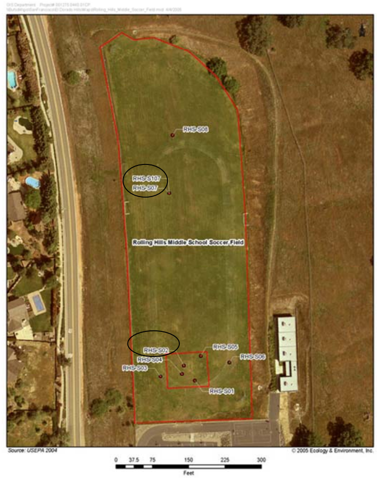
Figure 5-22 Rolling Hills Middle School Soccer Field Soil Sample Locations
